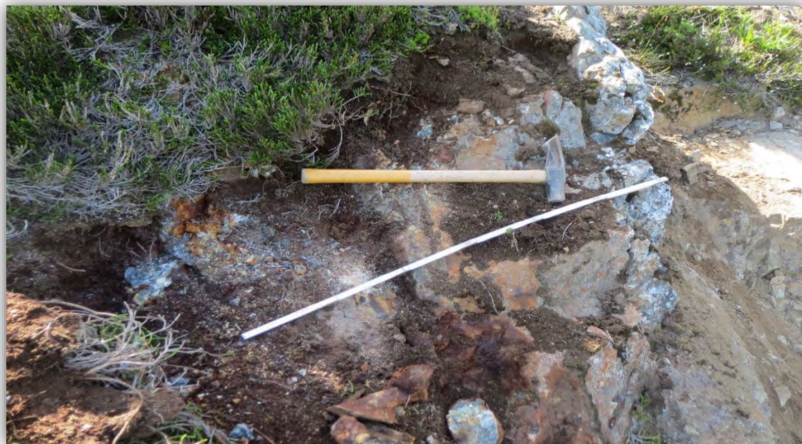
Mineralized Quartz Vein Breccia Along NW Margin of Felsic Dyke; Sample 749572 – 1.1 g/t Au, 392 ppm Ag
